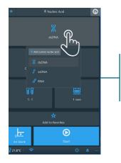
Built-in protocols allow accurate quantification of nucleic acids (dsDNA, ssDNA, RNA, or custom) using the Thermo Scientific  $\mu$ Drop Plate, microplates, or cuvettes.
