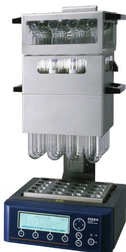
The lift eliminates heavy handling.
